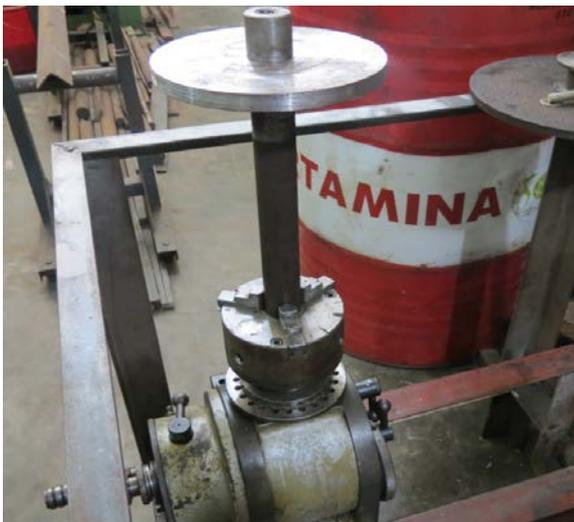
Gambar 4. *Fixture* benda kerja
