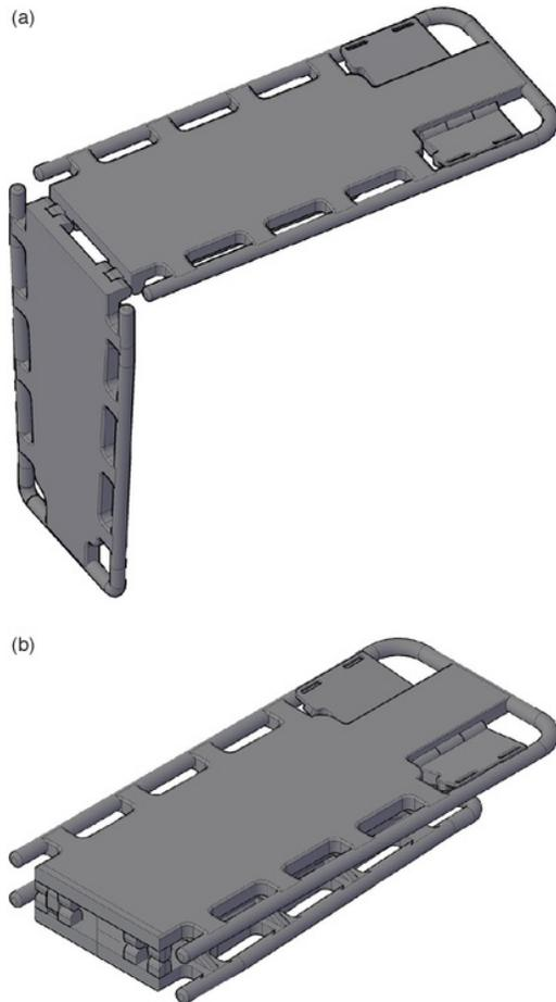
Figure 3. Fold in the spinal board.
