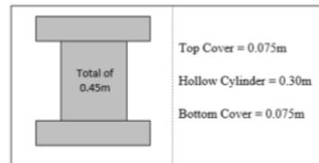
**Fig. 2** The StormPav GP Components
