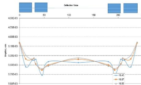
**Fig. 6** Surface deflection with different tire pressure (Rigid Pavement)
