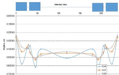
**Fig. 7** Surface deflection with different tire pressure (StormPav GP)
