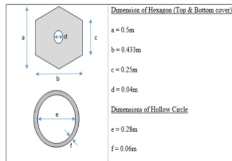
**Fig. 3** Details of construction of StormPav GP
