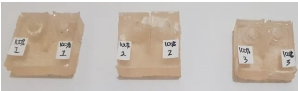
Fig. 6. Sample model test result mold crack test.
