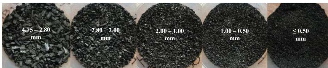
**FIGURE 2.** Morphology of biochar particle size from Surian (*Toona ciliata*) wood waste
