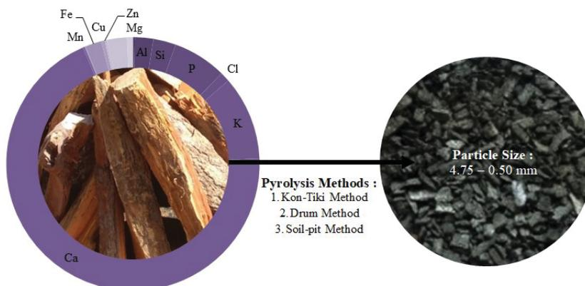
**FIGURE 1.** Wood waste to biochar (WTB) from Surian (*Toona ciliata*) as an ameliorant.
