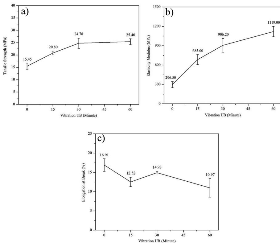
Fig. 5. Comparison of mechanical properties of all tested samples as function of duration vibration for (a) tensile strength; (b) elasticity modulus; (c) elongation at break.
