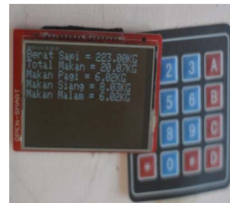
Fig. 17. Cow weighing's result and calculating feed in a day
