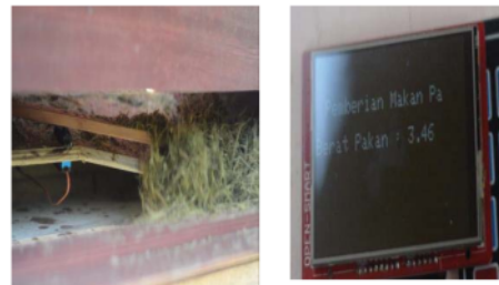
Fig. 18. The distribution process for breakfast (a) feed distribution for lunch by motor servo (b) result of reading distributed feed's weight
