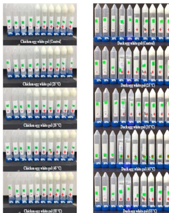
Figure 1: Tube inverting test using different concentrations and temperatures of control and ultrasound-treated chicken and duck egg white.
