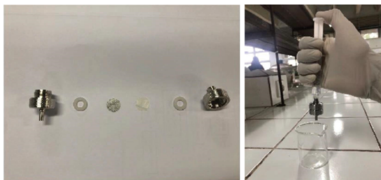
FIGURE 3: The filtration process of samples by NCB with filtration apparatus.
