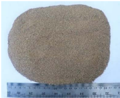
Fig.3 Combination of 70% sand + 30% clay
