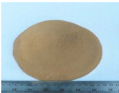
Fig.3 Combination of 70% sand + 30% clay
