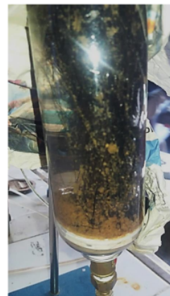
Figure 9. Anammox bacteria growth as biofilm in the palm fiber.
