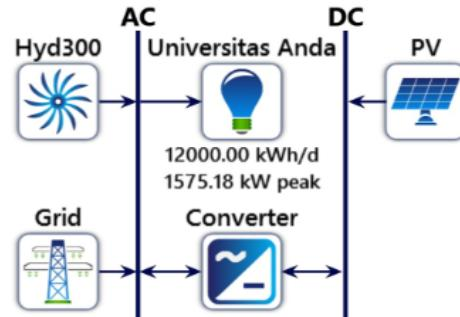
Fig 4. Schematic diagram of the MH-PV grid system
