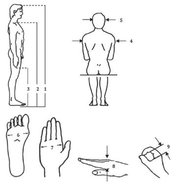
Figure 6. Anthropometric dimensions. Note: 1 =stature; 2 =shoulder height; 3 =fingertip height; 4 =shoulder breadth; 5 =head breadth; 6 =foot breadth; 7 =hand breadth; 8 =hand thickness; 9 =grip diameter.
