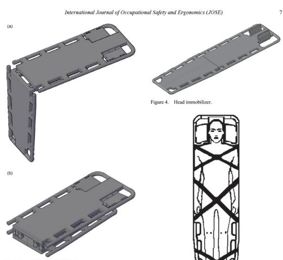
Figure 3. Fold in the spinal board. Note: (a) Spinal board in the unfolded state; (b) Spinal board in the folded state.
