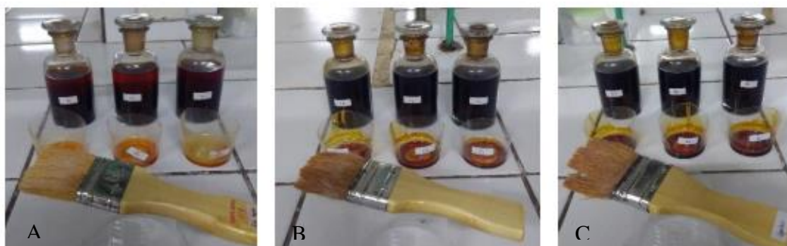
Figure 1. The appearance of produced varnish from ambalau resin extracted with methanol (A), ethanol (B) dan acetone (C).
