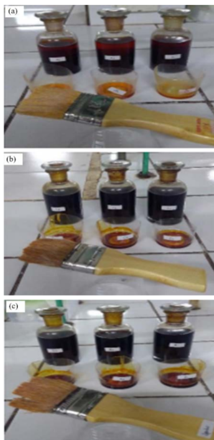
Fig. 1(a-c): Appearance of produced varnish from Ambalau resin extracted with (a) Methanol, (b) Ethanol and (c) Dan acetone
