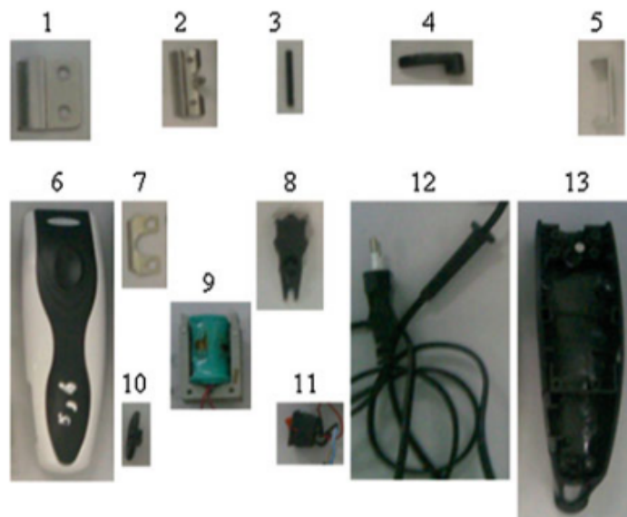
Fig. 2 Hair clipper. 1 Low cutter, 2 Upper cutter, 3 Tip, 4 Handle, 5 U-shape, 6 Upper cover, 7 Front part, 8 Magnet, 9 Coil, 10 Outer switch, 11 Inner switch, 12 Cable, 13 Lower cover
