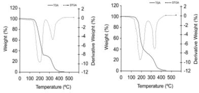
Fig. 11. TGA Thermogram of PS - Starch Blend<sup>31</sup>
