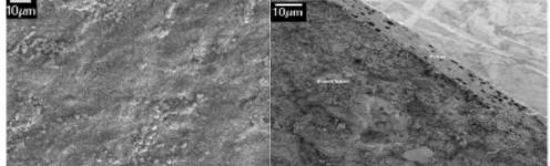
Fig. 4. Surface and Cross-section of PS - PU Coated Urea<sup>11</sup>
