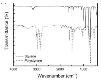
Fig. 3. Example of FTIR Spectrum from Polystyrene and Styrene<sup>16</sup>
