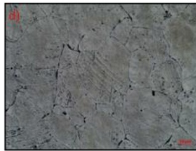
Figure 4. The microstructure of Mg-0.7%Ca alloy forged at (a) 140°C, (b) 180°C, (c) 220°C, and (d) 260°C at the speed of 25spm.
