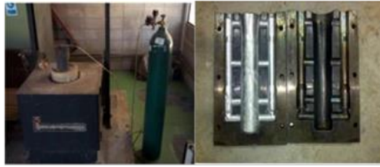
Figure 2. Induction furnace and steel mold
