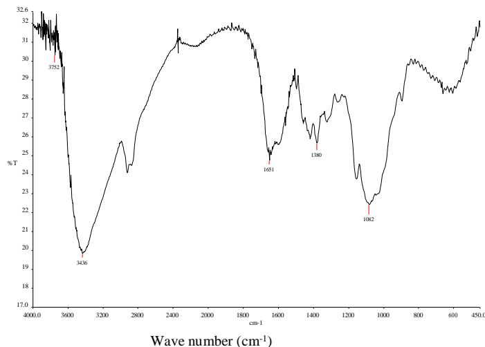
Fig 2(a). Infrared spectrum of standard chitosan (Chitosan SIGMA®) in a KBr plate.
