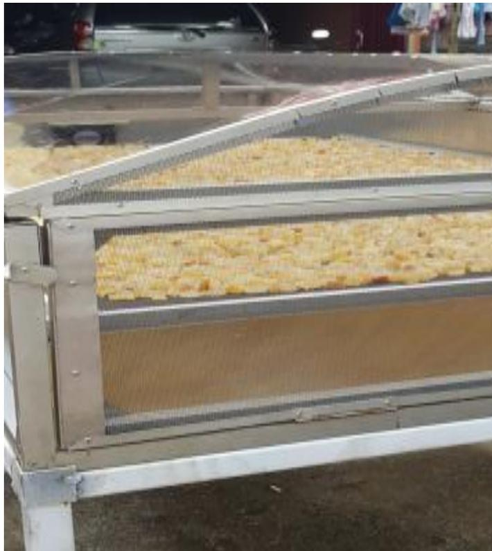
Gambar 7.5. Solar Tunnel Dryer.
