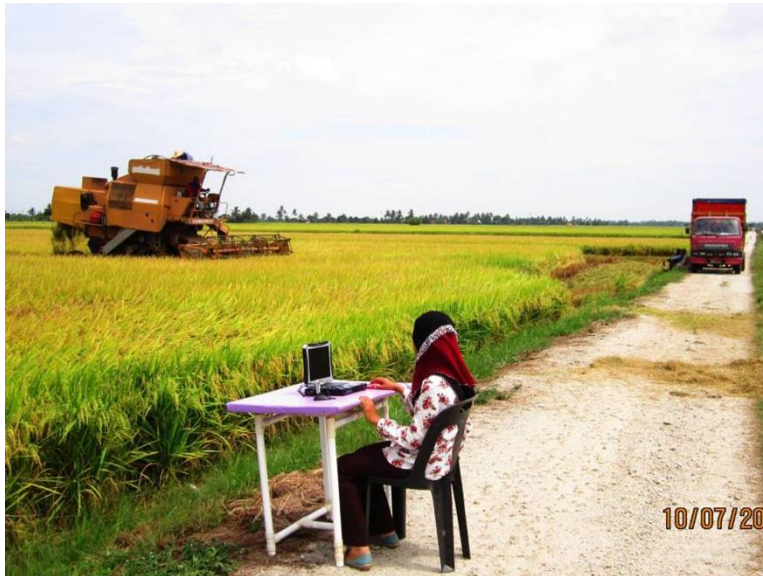
Fig 1. Monitoring instantaneous yield at on-ground workstation with the instrumentation system on-board the come.
