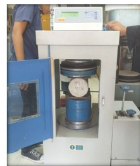
Fig. 5 Splitting tensile test on cylindrical specimen
