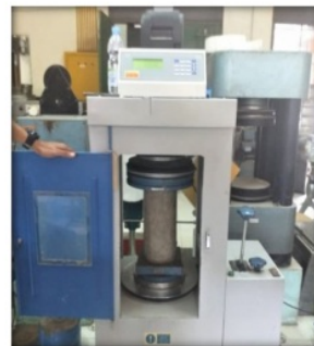
Fig. 4 Compressive test on cylindrical specimen
