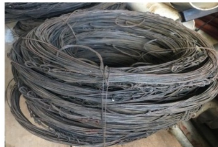
Fig. 2 Steel wires from waste tyre
