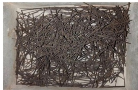
Fig. 3 Steel fiber waste tyre ( \pm 4 cm length)
