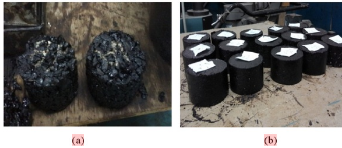
Fig. 2. (a) Porous Asphalt Sample (b) Asphalt Concrete Sample
