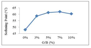
Figure 3: Softening Point of various Gondorukem in Bitumen
