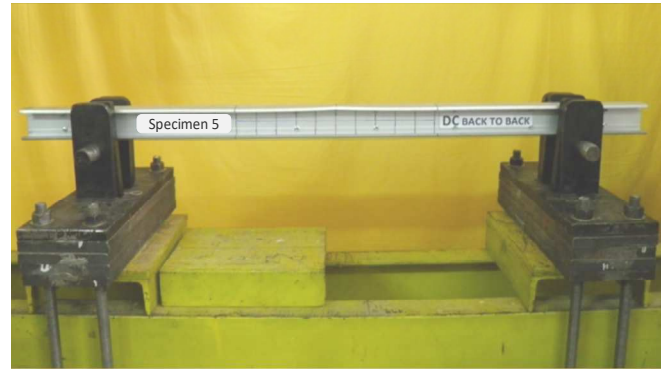
Fig. 5 Elastic lateral buckling on DC-I: deformed beam (left) and beam returned to its original position after load removed (right)
