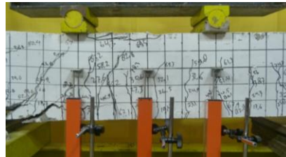
(b) Typical failure after test.
