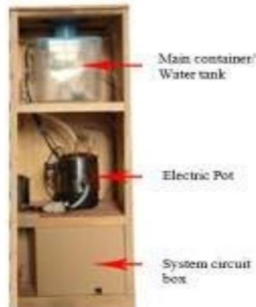
Figure 5. Overall dispenser heating system
