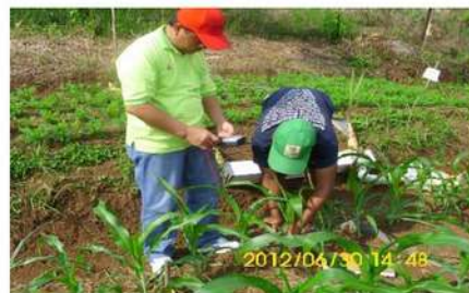
Figure 1 Photo measurements of soil water con-tent with gypsum blocks and ohm meter on a swath of the experiment.
