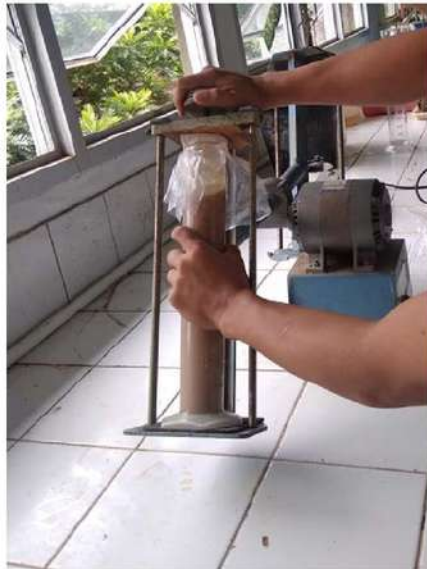
Fig 4. Dust fraction analysis using a shaker
