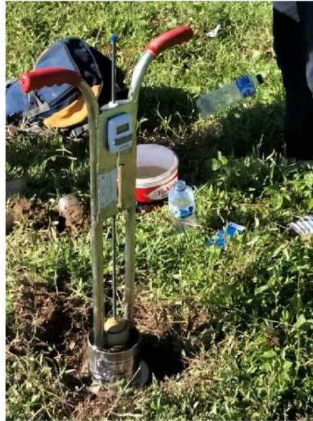
Fig. 2 Measuring soil infiltration capacity on the field
