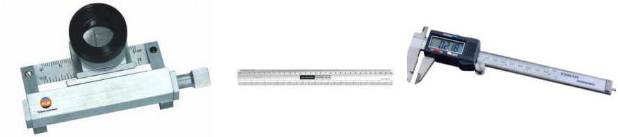
Gambar 2. Alat ukur paper point a: Calibrated magnifying glass , b: transparent scale , dan c: digital caliper (Hefei Fanyuan Instruments Co. Ltd, Cina).
