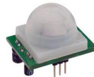
Gambar 2.3.1. Sensor *Passive Infra Red (PIR)* [14]
