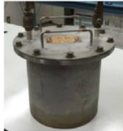
Fig. 2. The oil tank used for the thermal aging test.
