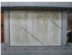
Photo 6. Initial Damage to Infilled Wall
