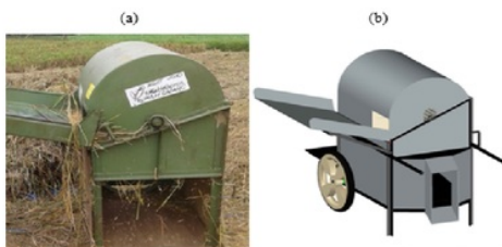
Fig. 9 The Funnel Form where the Rice Fell Out- Former Design (a) New Design (b)
