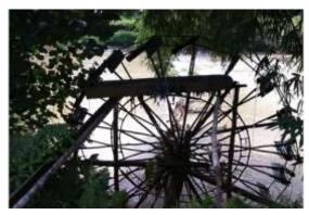
Figure 2 Traditional watermills to bring water up from Momongan river into rice field in IX Koto Dibauah, Dharmasraya Regency,(*yf-doc.2016*)
