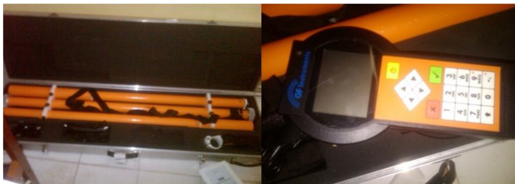
Gambar 2. GF Instrument CMD-4: (a) 3 buah probe, (b) main unit
